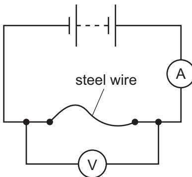
The reading on the voltmeter is 1.50 V and the reading on the ammeter is 4.90 A.
