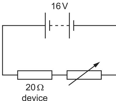
The power dissipated in the electrical device is 4.0 W.
