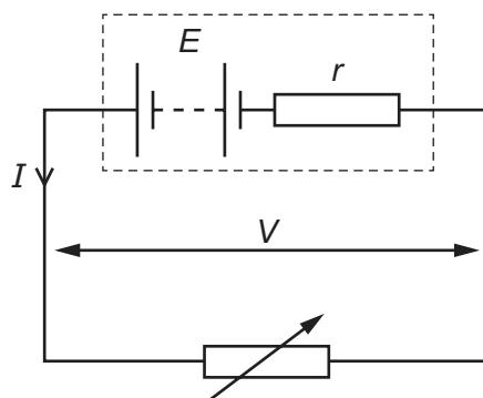
The variable resistor is adjusted so that  $I$  increases.
